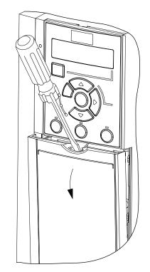
Illustration 1.2 Removing the Front Cover of the Frequency Converter
