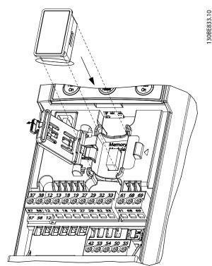
Illustration 1.4 Plugging the Memory Module in the Frequency Converter
